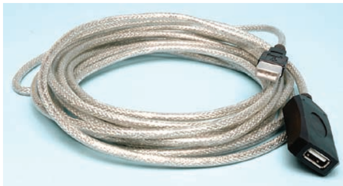
This active USB 5m extension cable uses some of the power available from the USB port to amplify the data signal. Up to five can be connected in series.
