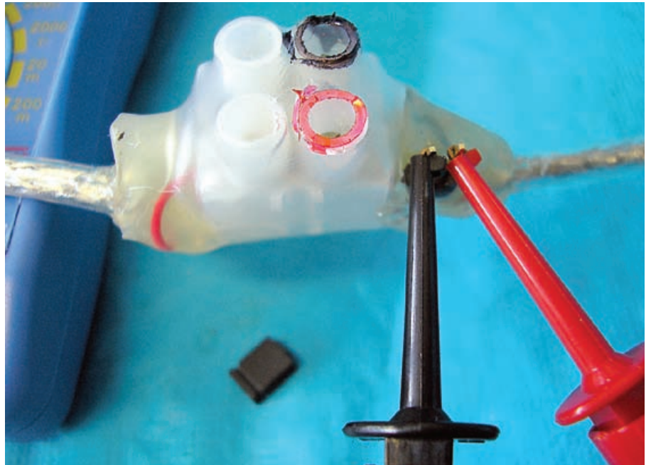
Here's Stan's prototype USB breakout 'box', potted in some hot-melt glue. The idea is to poke your multimeter probes into the terminal block (avoiding shorts) for voltage measurements; for current measurements, you remove the header pin shorting block and connect your multimeter in series.
