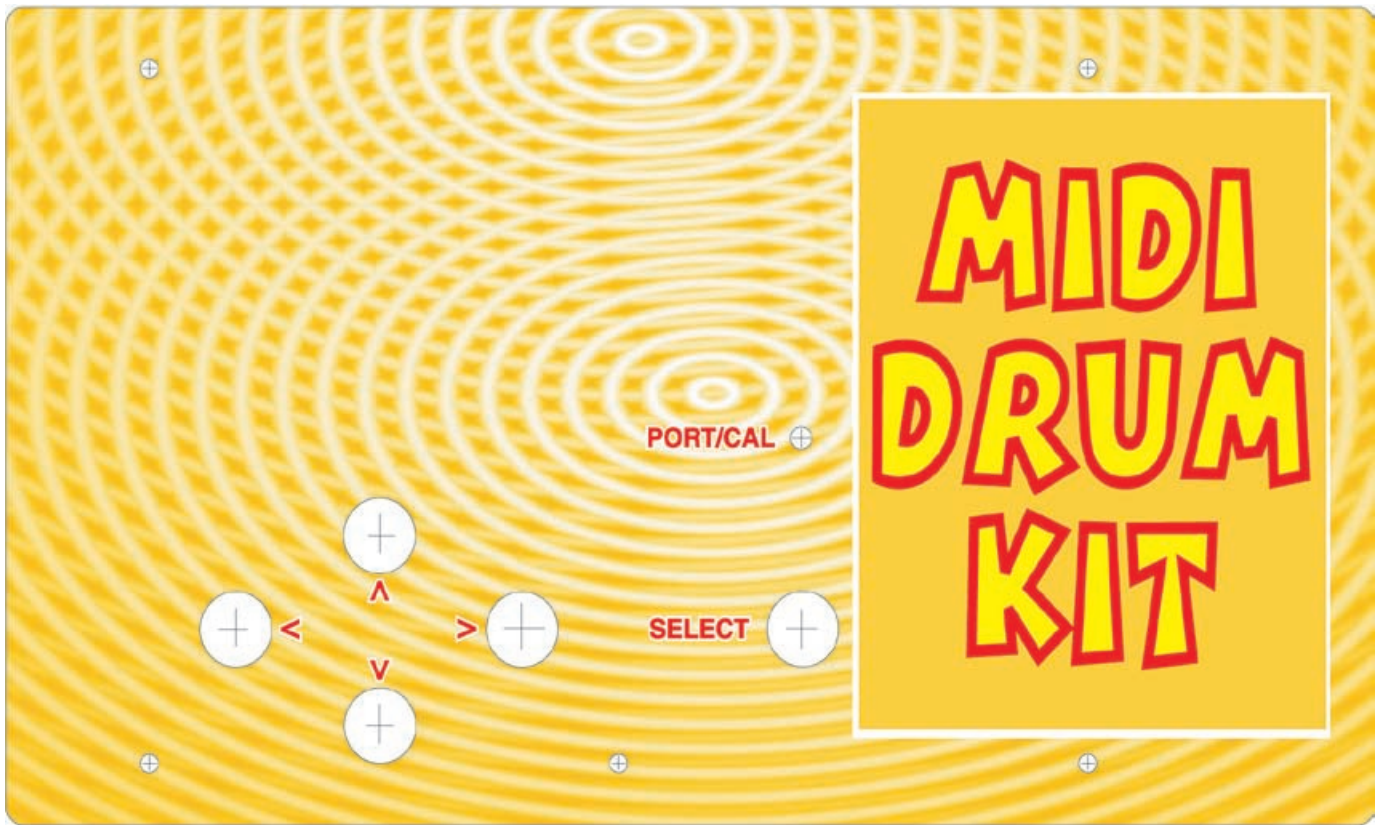
Fig.4: the full-size front panel artwork with hole positions for the switches and mounting holes. No display cutout is shown as this will vary with the type of display. An accurate photocopy of this could also be used as a drilling template.
