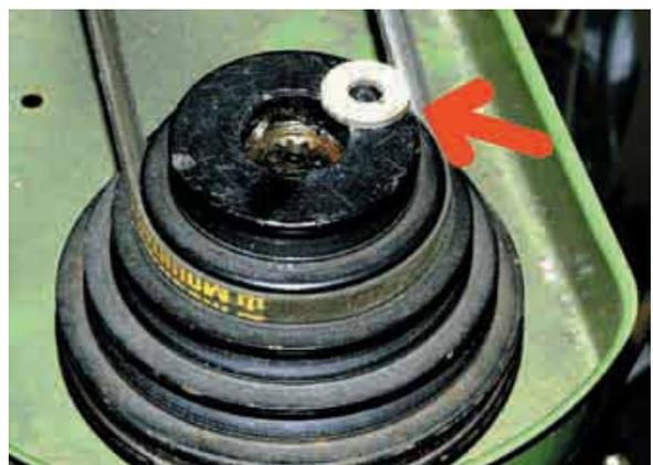
The reed switch is triggered by this magnetic washer which is glued to the pulley. This washer was extracted from a salvaged stepper motor.
