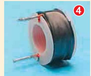
Above: these photos show how to make a simple jig from scrap material to wind the 6.8 $\mu$ H inductors (see text). First, the bobbin is slipped over the collar on the bolt (1), then the end cheek is attached and the wire threaded through the exit slot (2). The handle is then attached and the coil wound using 25.5 turns of 1mm enamelled copper wire (3). The finished coil (4) is secured using a couple of layers of insulation tape and a band of heatshrink tubing.
