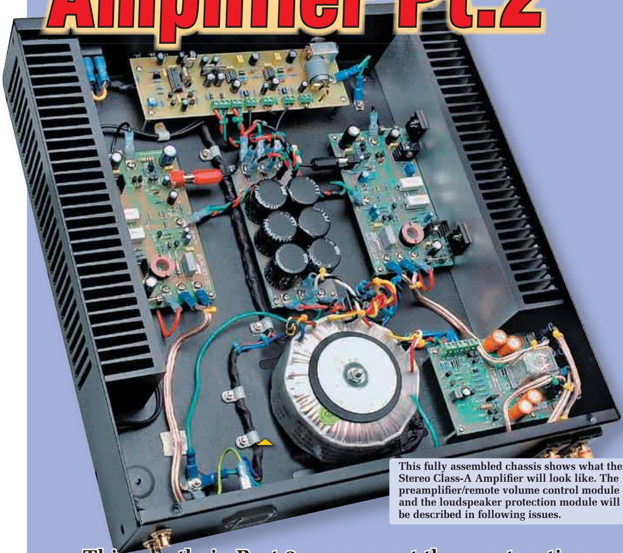
This fully assembled chassis shows what the Stereo Class-A Amplifier will look like. The preamplifier/remote volume control module and the loudspeaker protection module will be described in following issues.
