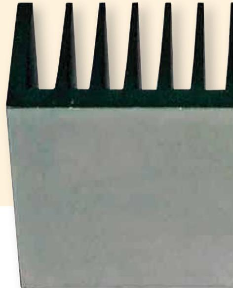
Here's another view of the fully-assembled right-channel power amplifier module, attached to its heatsink. After mounting the output transistors, it's a good idea to use a multimeter (set to a high ohms range) to confirm that they are correctly isolated from the heatsink. You should get an open-circuit reading between the heatsink and each of the transistor leads.
