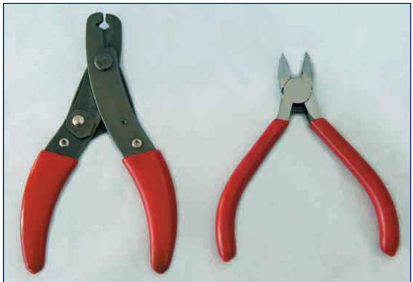
Fig.1. Proper wire strippers and cutters are essential tools for project construction, and an inexpensive combination tool (left) does both jobs quite well. It is also worthwhile augmenting these with a small pair of cutters (right) for intricate work and for cutting fine wires
