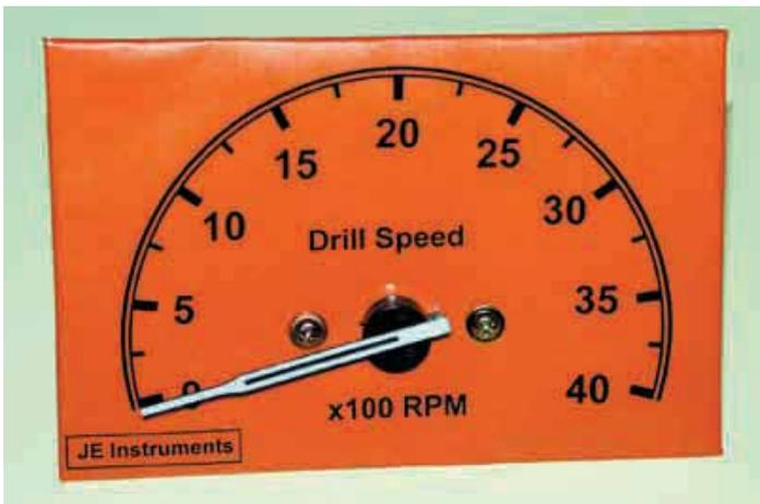
The revised and modified scale, printed out on orange paper and covered in clear self-adhesive film. But just who is behind the 'JE Instruments' company?
