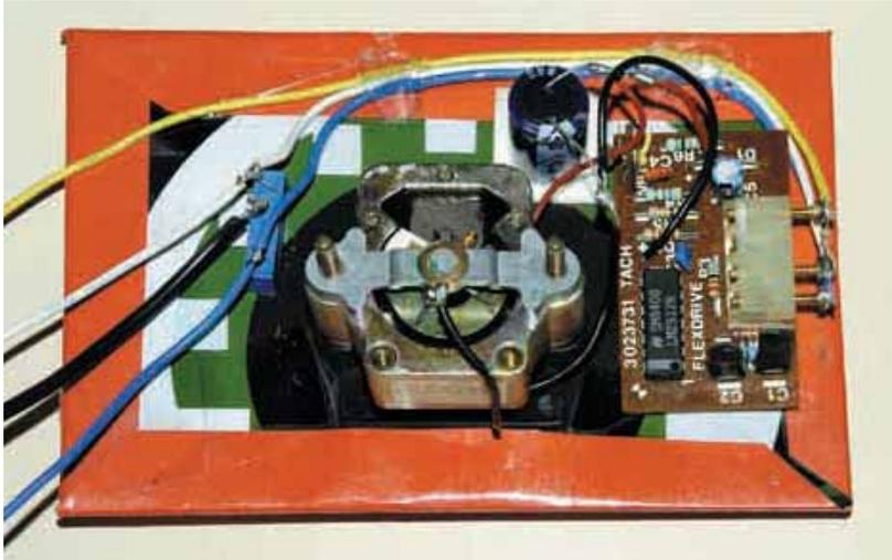
The rear of the modified assembly. At left is the pot providing the +5V reed switch supply, at top-right is the new smoothing capacitor, and at right is the PC-board from the original tachometer. The 33kΩ pull-down resistor is just visible at far right and connects the signal input to ground.
