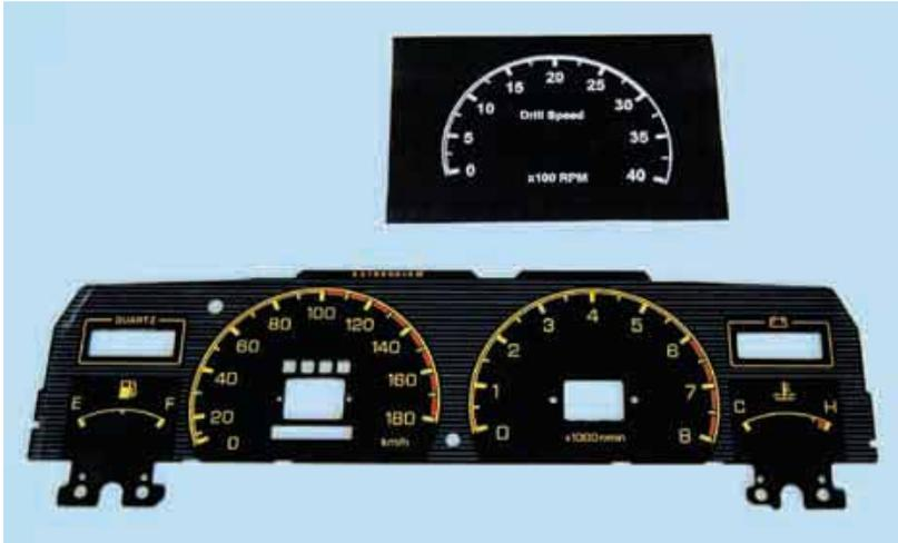
Here's the original instrument panel and an early draft of the scanned and re-scaled drill press tacho scale. It's printed out 1:1 and so is a perfect size match for the original instrument.
